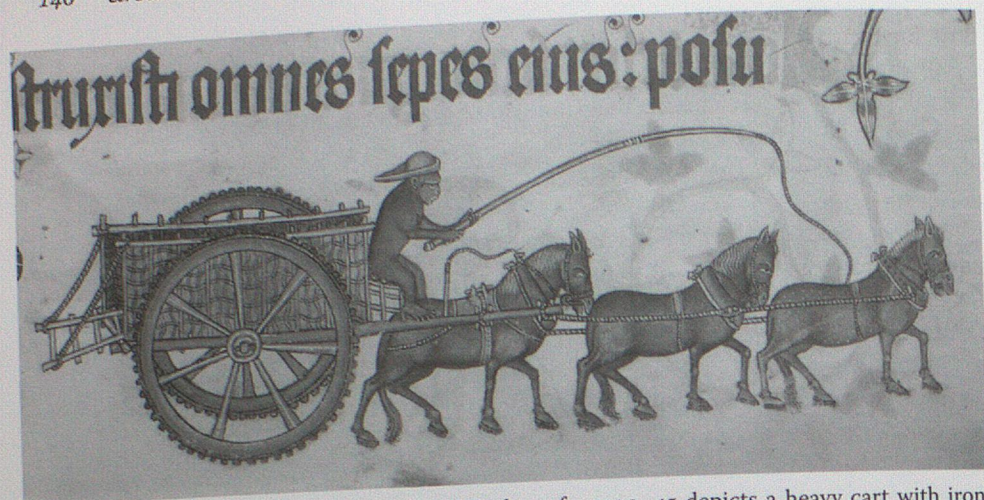
7 An engaging illumination from the Luttrell Psalter of c. 1320–45 depicts a heavy cart with iron-bound wheels, of the kind so often banned from late medieval cities. The studded nails used to attach the metal rims to the wood improved traction, but caused great damage to paved streets.
